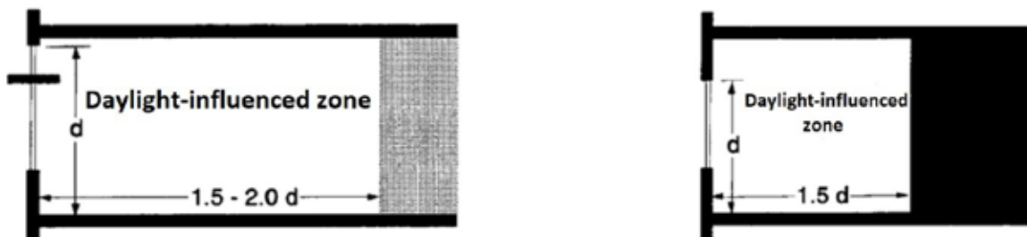
Fig. 1. Standard daylight penetration depth for south-facing windows: 1.5 times the window head height for conventional windows and up to 2 times with a light shelf. Source: Luther, 2004.
