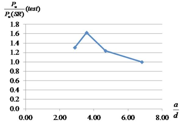
Fig. 11: Effect of shear span to effective depth ratio on flexural strength of slab specimen (Series I). Source: Authors.
