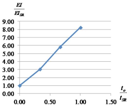
Fig. 12: Effect of overlay thickness on flexural stiffness. Source: Authors.
