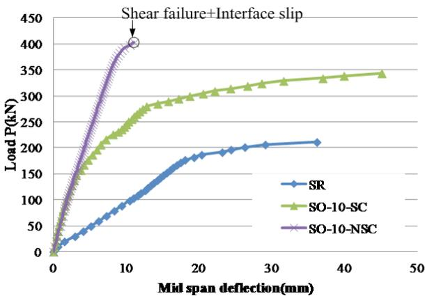
Fig. 8: Relationship between load and mid-span deflection of test series II. Source: Authors.
