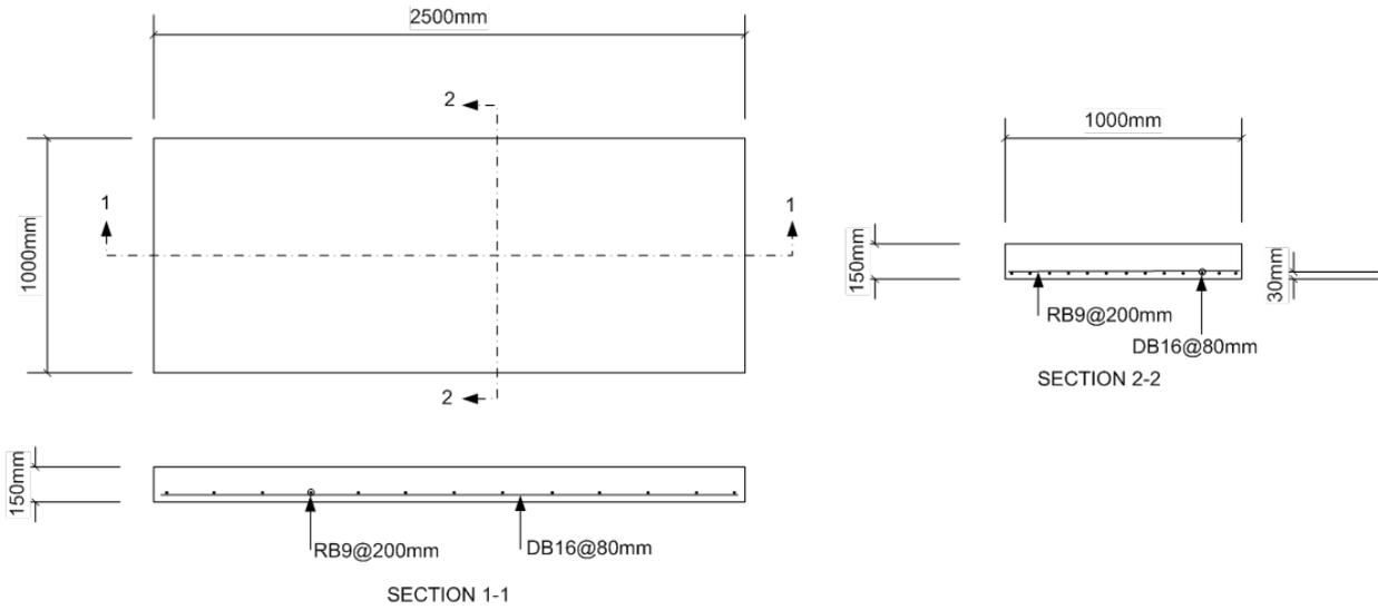
Fig. 2: Details of reference slab specimen. Source: Authors.
