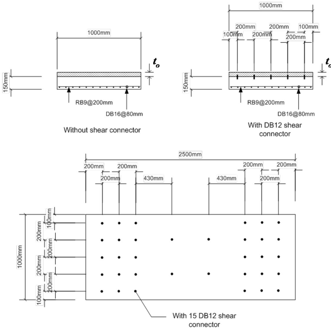
Fig. 3: Details of slab specimen with overlay and with or without shear connectors. Source: Authors.
