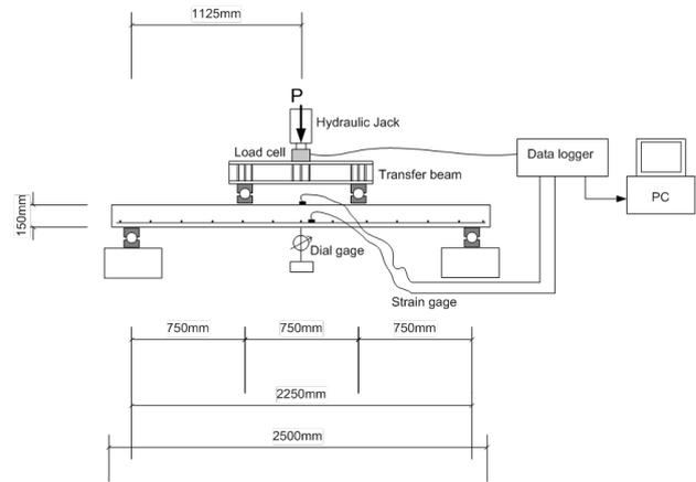
Fig. 5: Test set up of slab specimen
