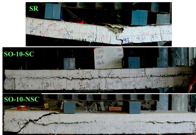
Fig. 9: Failure mode of the second test series. Source: Authors.
