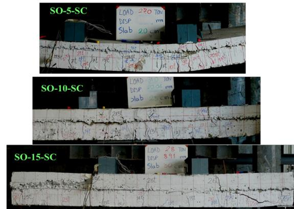
Fig. 7: Failure mode of the first test series.
