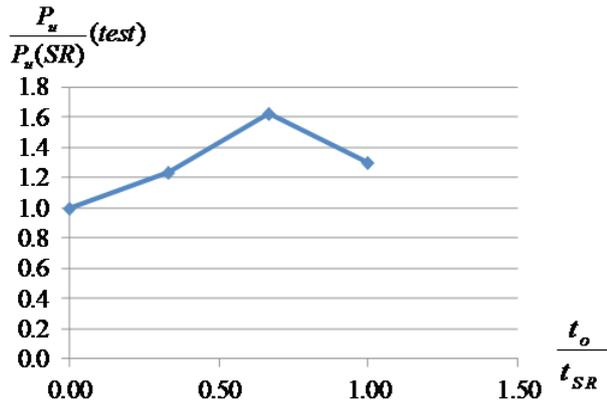
Fig. 10: Effect of overlay thickness on flexural strength of slab specimen (series I). Source: Authors.
