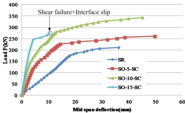
Fig. 6: Relationship between load and mid-span deflection of test series I. Source: Authors.
