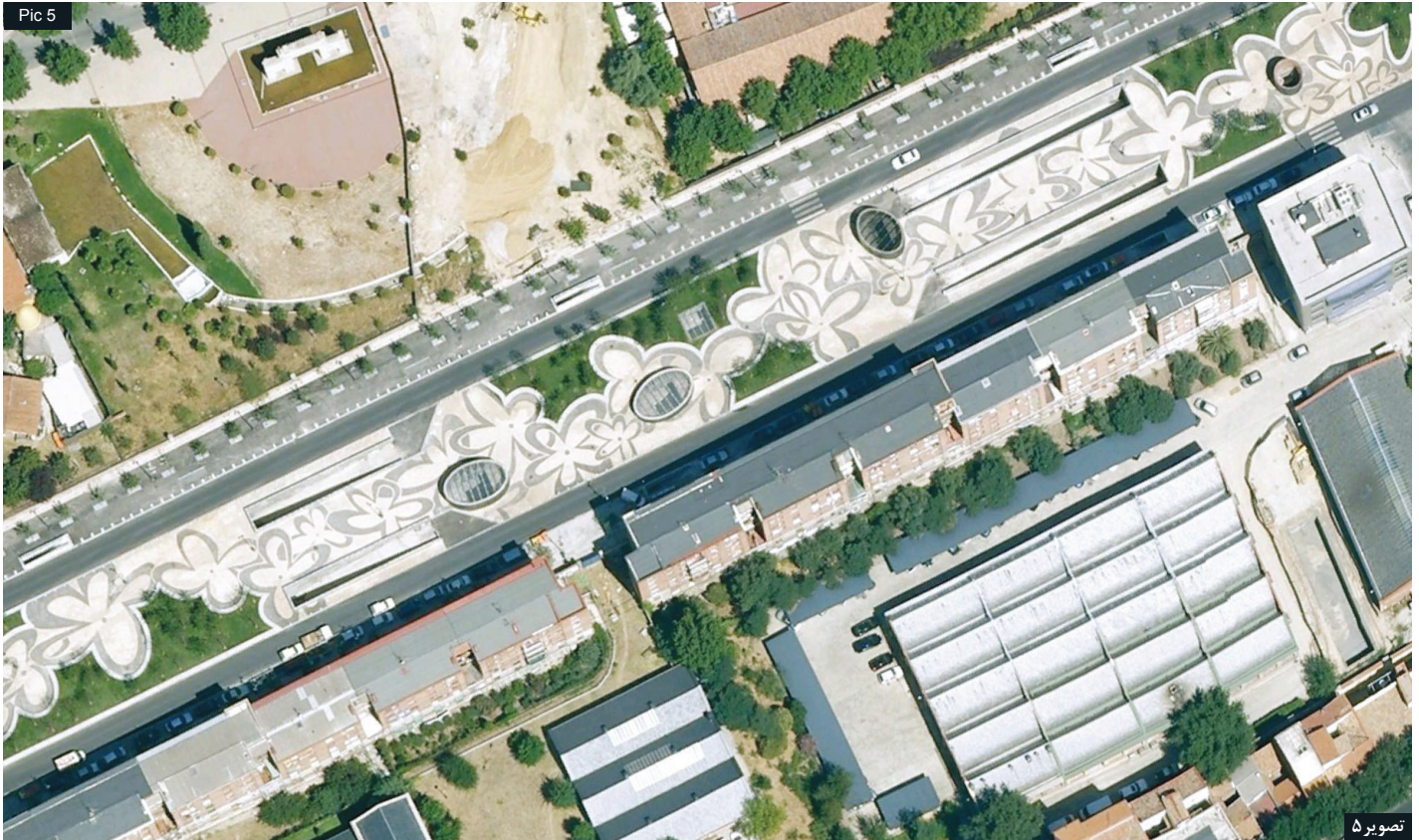
Pic5: zoomed aerial photo of "Avenida de Portugal" in 2010, using the underground tunnels as parking spaces with the capacity of 1000 cars, has transferred the street to a linear garden-street which is in direct interaction with citizens' lives. Source: www.maps.google.com .
