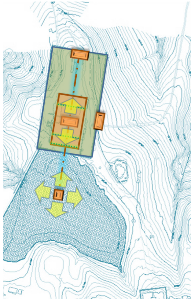
Fig. 8. The analysis of the plan of Abbasabad Garden; rectangular geometry, deep axis and terracing the garden; the placement of the semi-open pavilion at the highest point of the garden, the deep inner view and landscape and exterior views from the mansion to the lake and plain of Behshahr and Peninsula of Miankaleh. Source: Authors.
