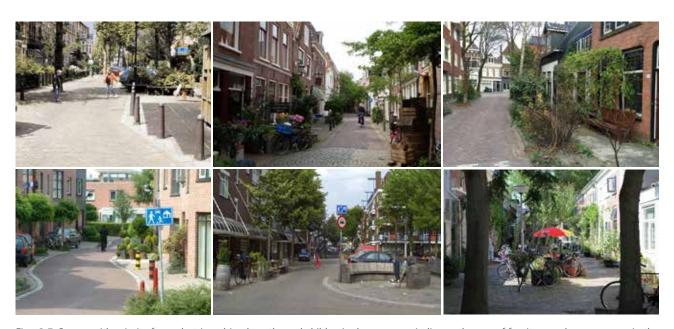
Figs. 2-7: Spaces with priority for pedestrians, bicycle paths and children's play spaces, winding paths, use of furniture and green spaces in the prototypical woonerf, Delft, the Netherlands. Source: www.feedyeti.com/woonerven.
